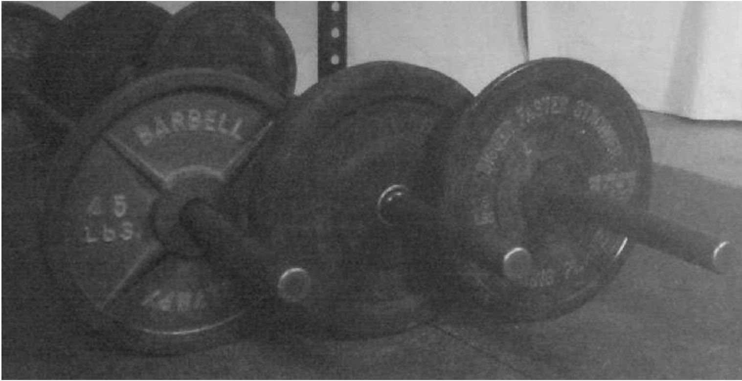
Figure 4-9. Standard plate diameter provides a standard height for the bar above the floor. Different weights in this standard diameter allow people of different strength levels to pull from this standard height, 8 1/2 inches or 21.5 cm between the bottom of the bar and the floor.
